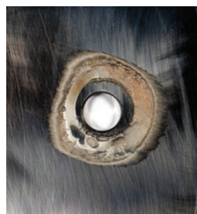
Samples tested for a week in saltwater under an applied potential of 300 mV. From left: Alloy 625 initiated crevice corrosion after less than 60 hours of exposure; untreated 316L stainless initiated crevice corrosion in less than an hour of exposure; 316L treated with the SAT12 process showed no initiation or signs of etching after more than 160 hours.
